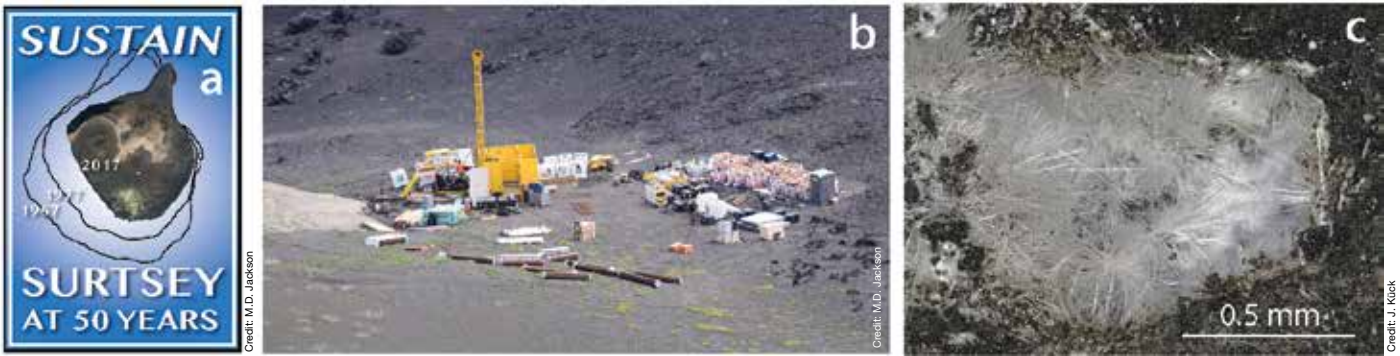
Figure 7. a,b) Surtsey volcano in Iceland is the location of the 2017 International Continental Drilling Program SUSTAIN project. c) Scanning electron microscope-secondary electron image of Al-tobermorite from SE-03 core at 124°C and a 147-m inclined depth.
